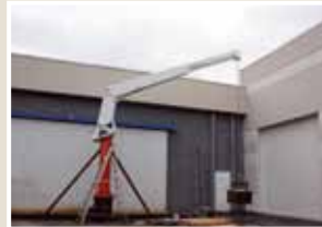
Cranes are proof tested to 110% of capacity
